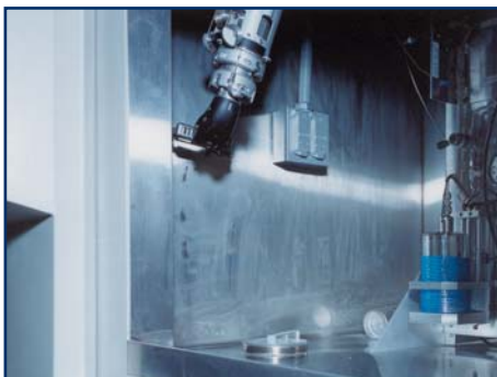
Hot cell with seamless stainless steel interior
